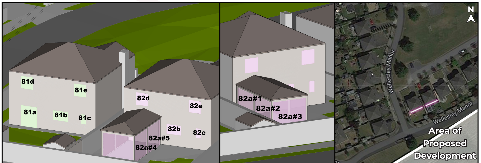
Figure 6.3: Left - Highlighted areas indicate the position of assessed windows., Right - Aerial view of assessed location
